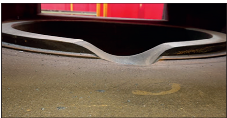
Erosion usually found without installation of patented baffle technology
